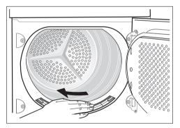
After a period of time, a gleam due to detergent residue on laundry forms on the filters. When this occurs, clean the filters with warm water using a brush. Remove the filter from the door pulling it out. (It can be positioned with the locating spur facing to the left or to the right).
